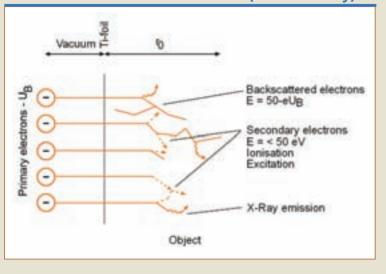
penetrate into the material with a range up to r<sub>0</sub>.
