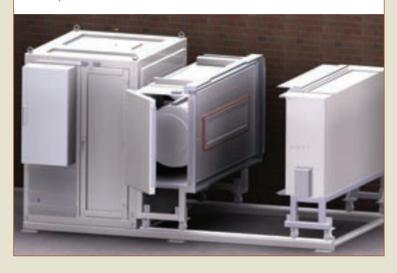
Its uncomplicated construction, combined with a control system for automatic process control, enables the operator to quickly and easily replace cathodes and exit windows without assistance from the supplier. Replacing worn parts requires less than one hour.
